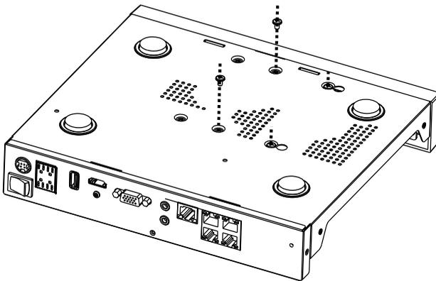
Step 5 Insert the hard disk data cable and power cable, then put on the upper cover and fasten the fixing screws.
